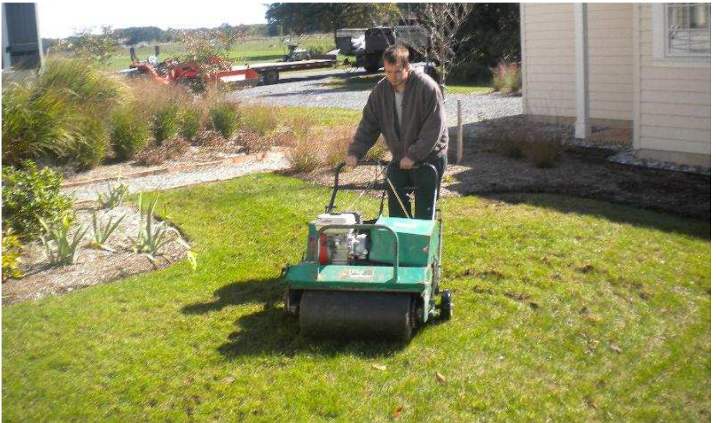
Jamie pushes one of our hand aerators. It's used for tight spaces when a tractor isn't needed.
